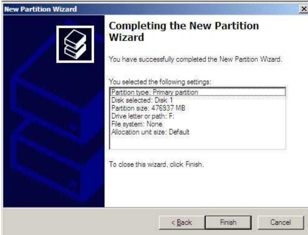
4. After the job above, the USB disk is formatted as a master partition. We need to formatted it as FAT32 file system so that it can be recognized by Vigor routers. We need to introduce a small tool here to do the job, fat32format.zip.
