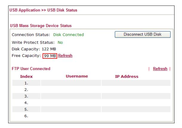
Note: If Write Protect Status shows Yes, it means you have turned on the write protect switch on the USB storage device and it is in read-only mode.
